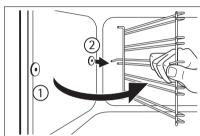
Installing the shelf support rails Install the shelf support rails in opposite sequence.
